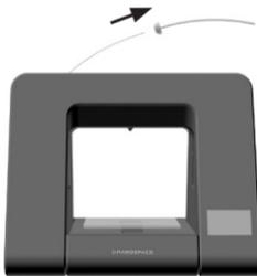
3. Insert filament through Teflon tube.
