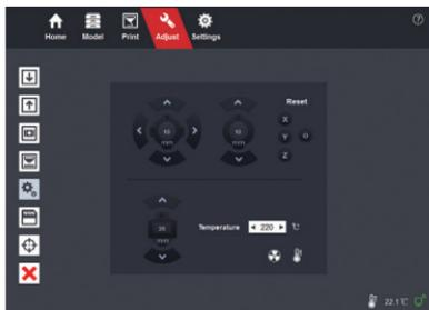
**Move on X, Y or Z direction:** Move the extruder left and right (X direction), move the print bed forward and backward (Y direction) and move the print bed up and down (Z direction).
