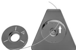
1. Open left filament holder cover and top lid, insert filament through the right hole on top of the filament holder.
