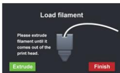
8. Click the “Finish” button after filament is extruded from the print head.
