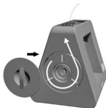
2. Place filament roll into the holder and close the filament holder cover.
