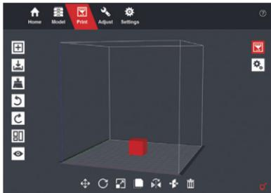
**Move selected models:** Move around the selected model in the print volume. Left column moves the model designated distance. Right column places the model to the designated point.
